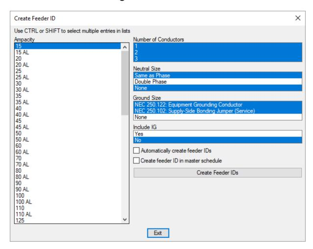
The **Create Feeder ID** dialog box is used to manually create one or more feeder IDs. Multiple settings can be selected to create feeder IDs for each combination of the selected settings.
