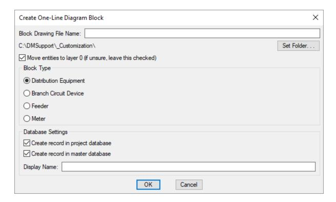
Block Drawing File Name: The name of the drawing file for the block.
