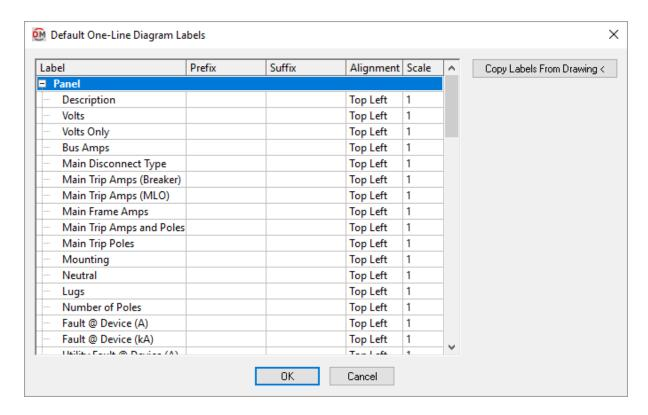
Copy Labels From Drawing: Press this button to copy the current label settings from an entity on the one-line diagram.
