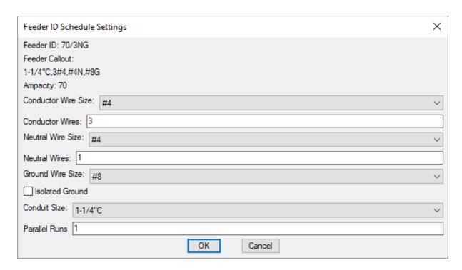
The **Feeder ID Schedule Settings** dialog box is used to change the wire size, number of wires, and other wire properties listed for the selected Feeder ID. These values are for informational purposes only and are not otherwise used.
